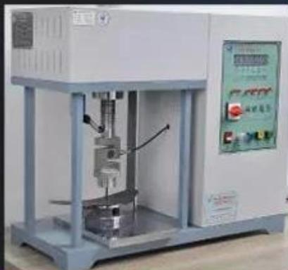
Midsole Test  $\geq 1200$  Newtons
