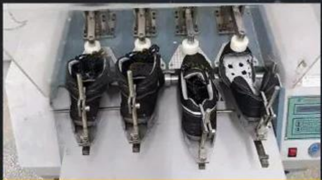
Flex Tester \geq 36,000 T
