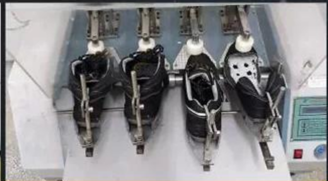
Flex Tester \geq 36,000 T
