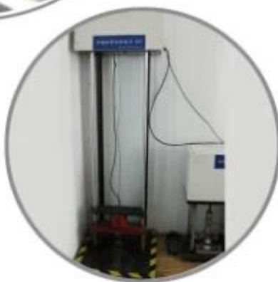
Impact Resistant Testing Machine
