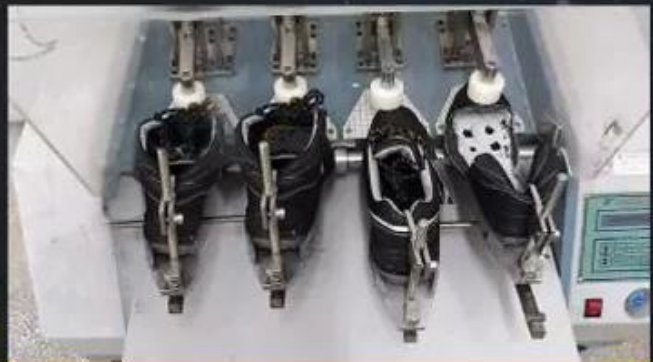
Flex Tester \geq 36,000 T
