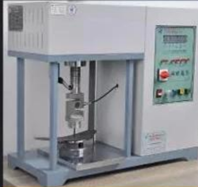
Midsole Test \geq 1200 Newtons
