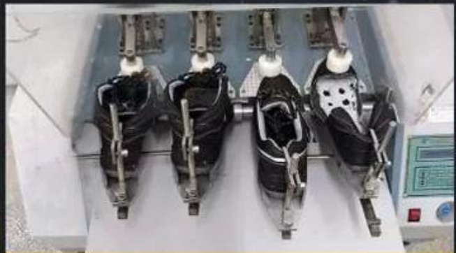
Flex Tester \geq 36,000 T
