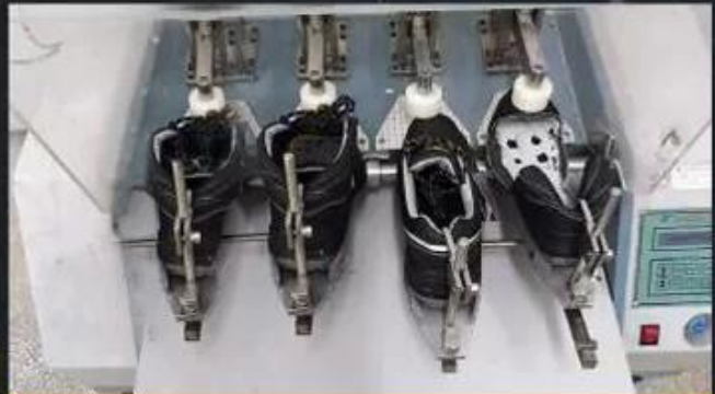
Flex Tester \geq 36,000 T
