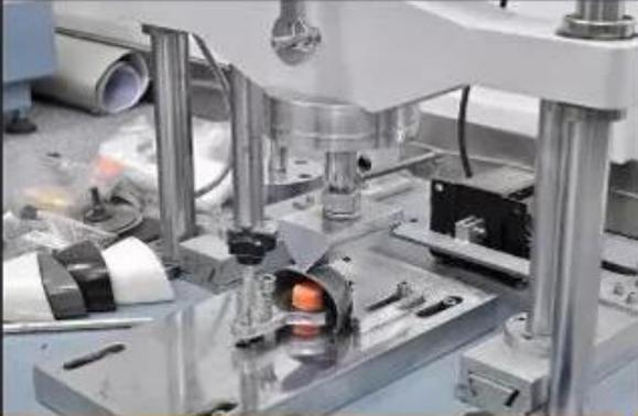
**Toecap Test  $\geq 200$  Joules**
