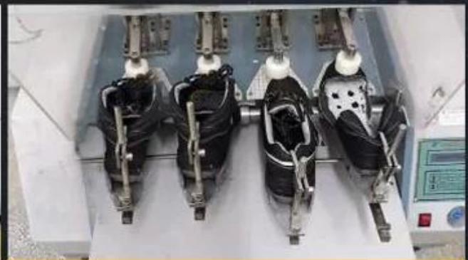
Flex Tester \geq 36,000 T
