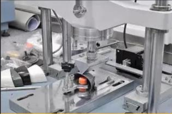
Toecap Test \geq 200 Joules
