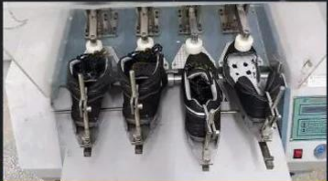
Flex Tester \geq 36,000 T
