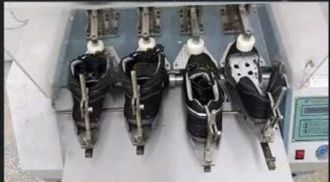
Flex Tester \geq 36,000 T
