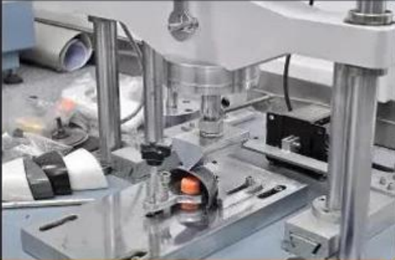
Toecap Test \geq 200 Joules
