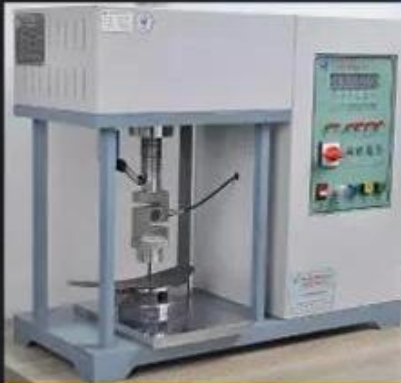
Midsole Test \geq 1200 Newtons
