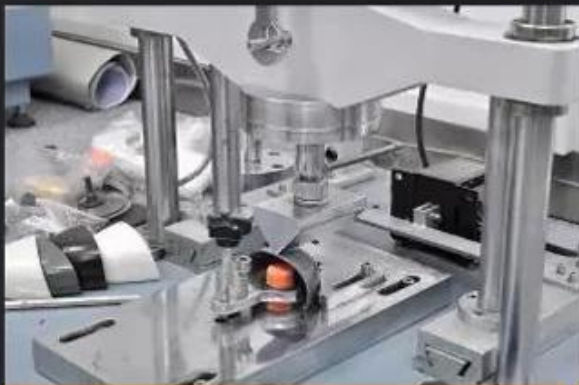
Toecap Test \geq 200 Joules
