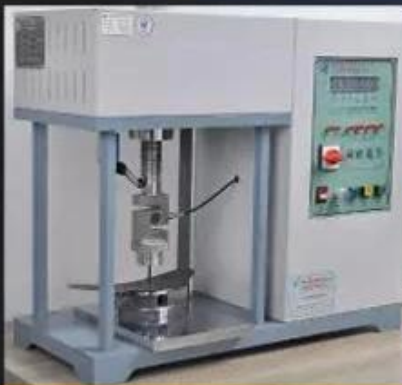
Midsole Test \geq 1200 Newtons
