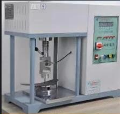
Midsole Test \geq 1200 Newtons
