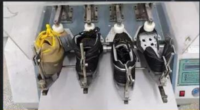
Flex Tester \geq 36,000 T
