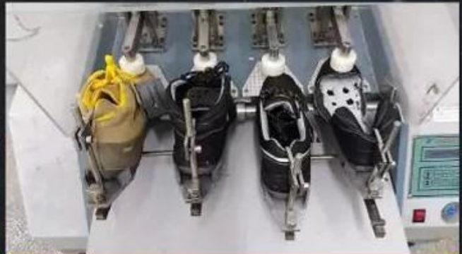
Flex Tester \geq 36,000 T
