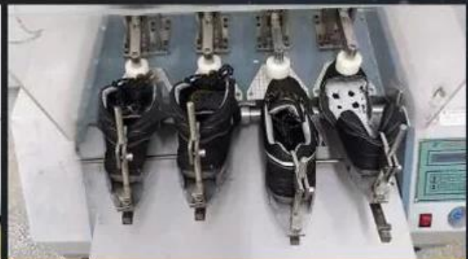
Flex Tester \geq 36,000 T
