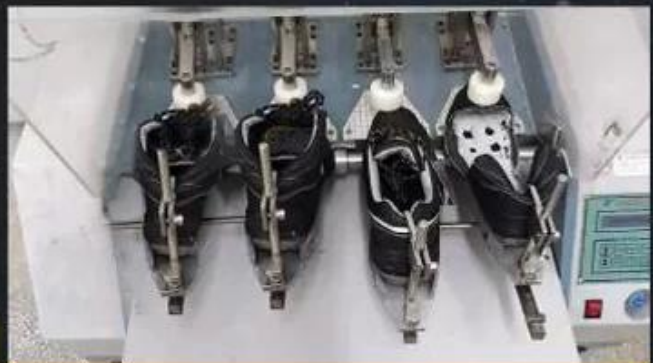
Flex Tester \geq 36,000 T
