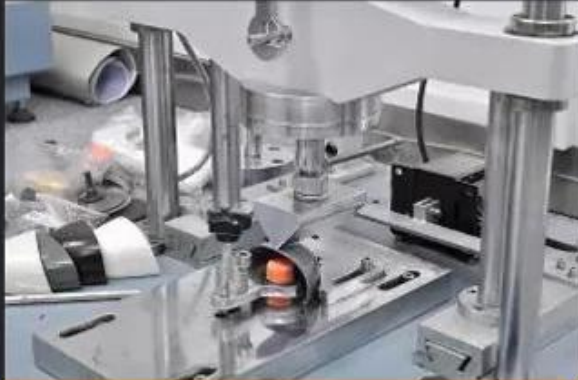
Toecap Test \geq 200 Joules
