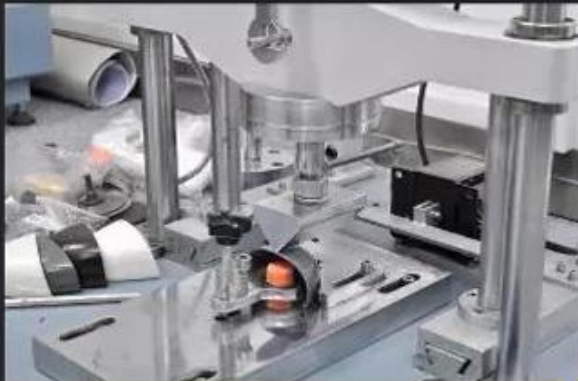
Toecap Test \geq 200 Joules
