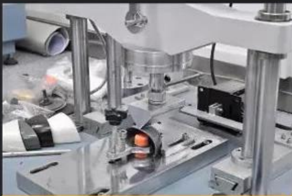
Toecap Test \geq 200 Joules
