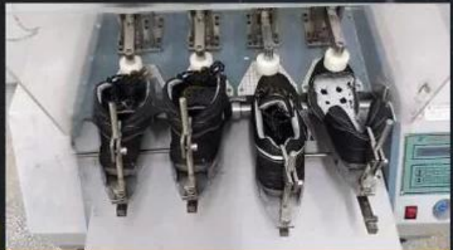
Flex Tester \geq 36,000 T
