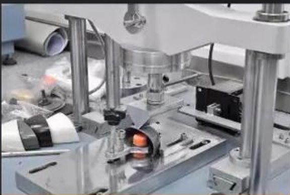
Toecap Test \geq 200 Joules
