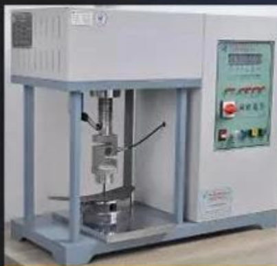
Midsole Test \geq 1200 Newtons
