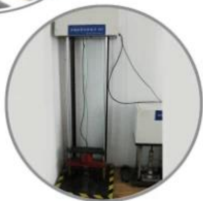
Impact Resistant Testing Machine
