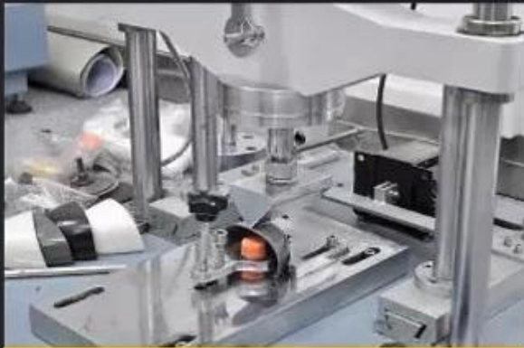
Toecap Test \geq 200 Joules
