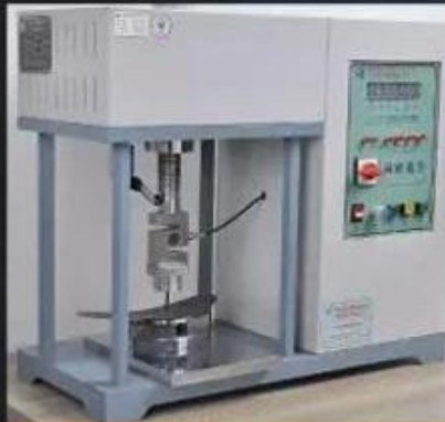
Midsole Test \geq 1200 Newtons
