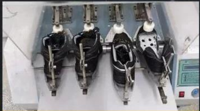
Flex Tester \geq 36,000 T
