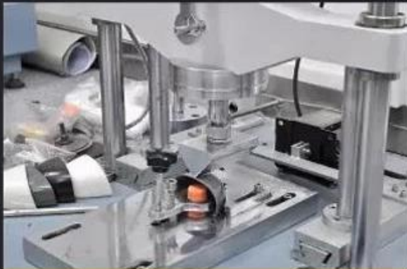
Toecap Test \geq 200 Joules
