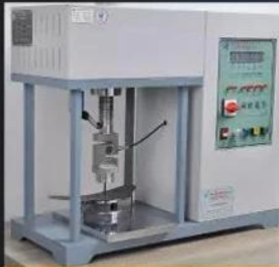
Midsole Test \geq 1200 Newtons
