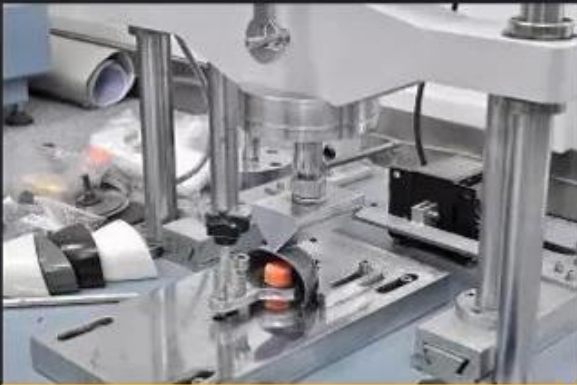
Toecap Test \geq 200 Joules
