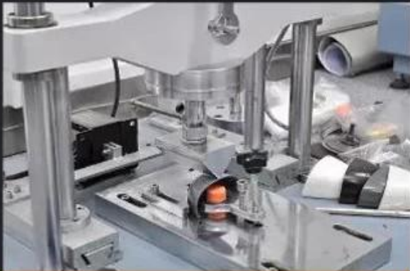
Toecap Test \geq 200 Joules
