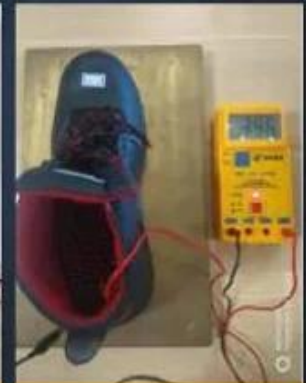
ESD Anti-Static Test
