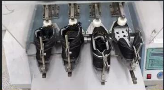
Flex Tester \geq 36,000 T
