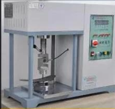
Midsole Test \geq 1200 Newtons
