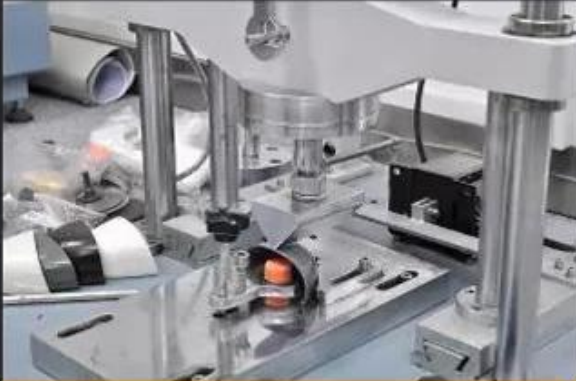
Toe cap Test \geq 200 Joules
