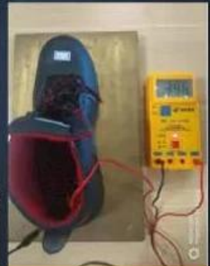
ESD Anti-Static Test
