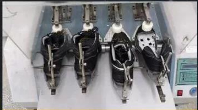
Flex Tester \geq 36,000 T
