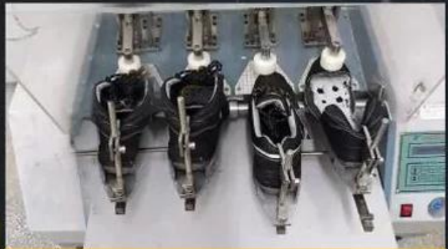
Flex Tester \geq 36,000 T
