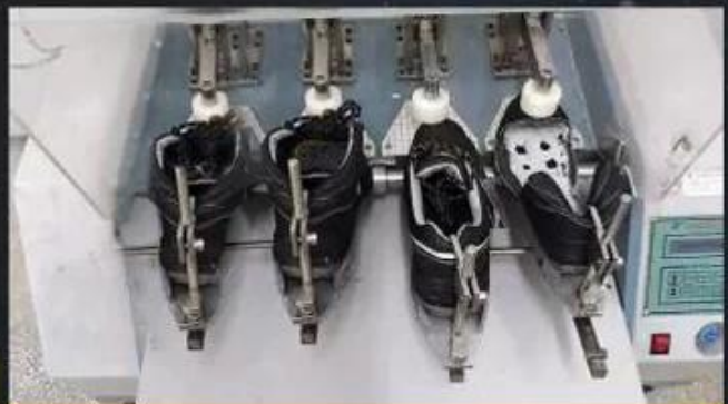
Flex Tester \geq 36,000T
