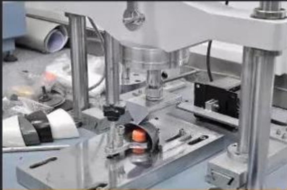
Toe cap Test \geq 200 Joules
