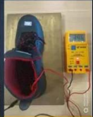
ESD Anti-Static Test
