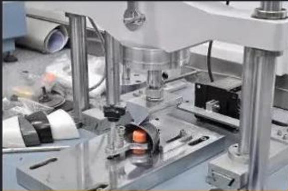
Toecap Test \geq 200 Joules
