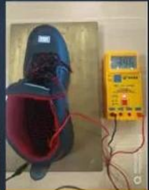
ESD Anti-Static Test
