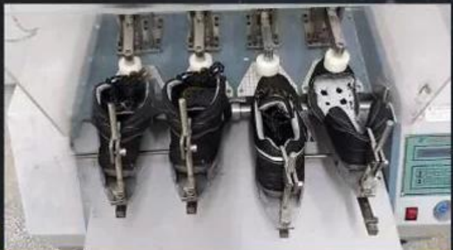
Flex Tester \geq 36,000 T
