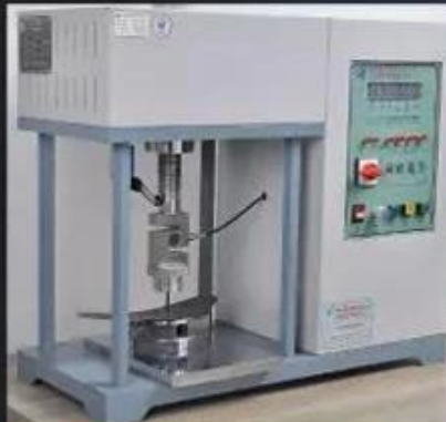
Midsole Test \geq 1200 Newtons
