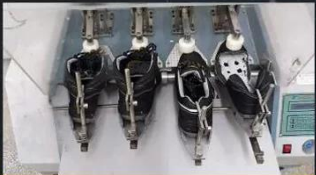
Flex Tester \geq 36,000 T
