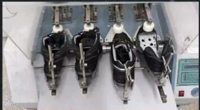
Flex Tester \geq 36,000 T
