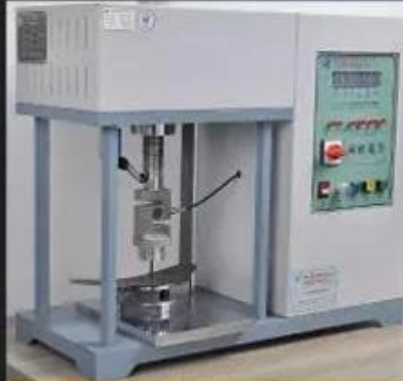
Midsole Test \geq 1200 Newtons
