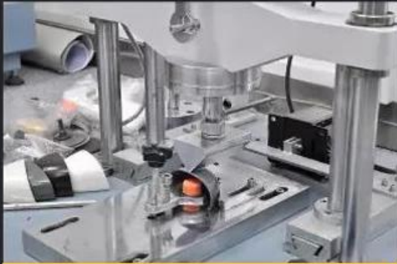
Toecap Test \geq 200 Joules
