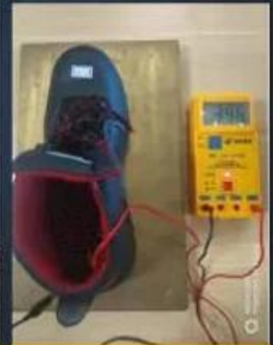
ESD Anti-Static Test
