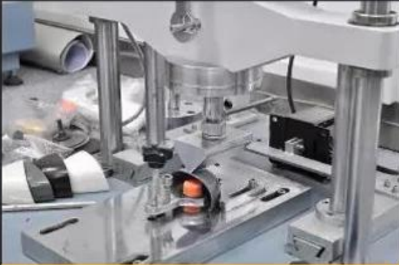
Toecap Test \geq 200 Joules
