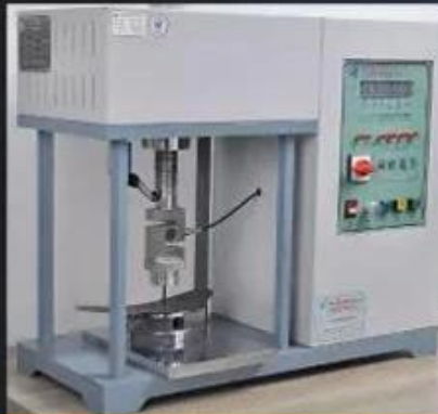
Midsole Test \geq 1200 Newtons
