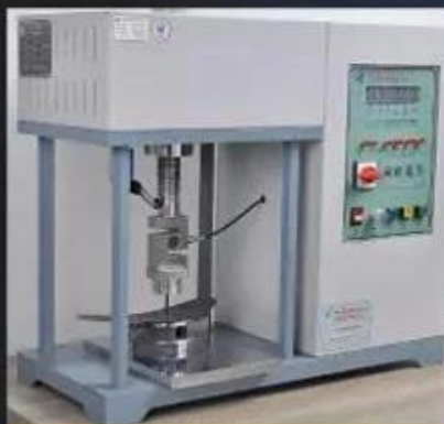
Midsole Test \geq 1200 Newtons
