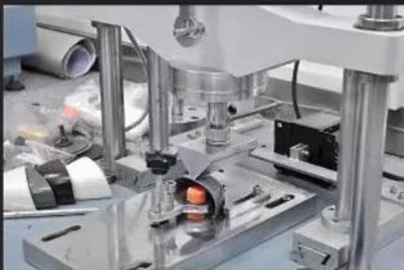
Toecap Test \geq 200 Joules
