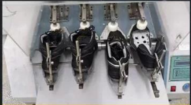
Flex Tester \geq 36,000 T
