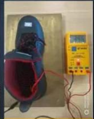
ESD Anti-Static Test
