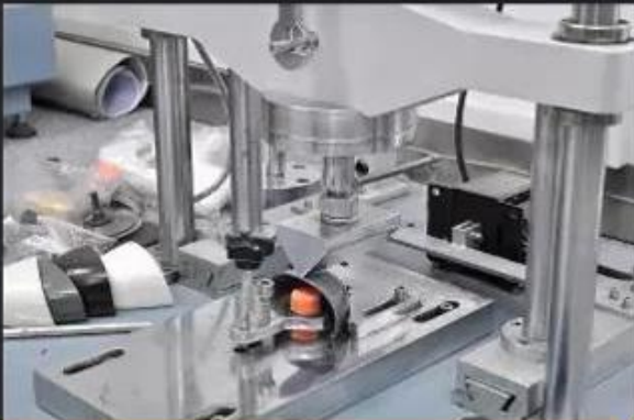
Toecap Test \geq 200 Joules
